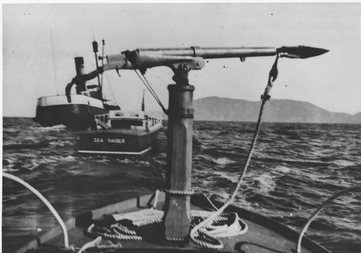
Fig. 17. Modern harpoon gun on a swivel base. Note the triple barb protruding from gun barrel; chaser and "Tuatea" in left background.
